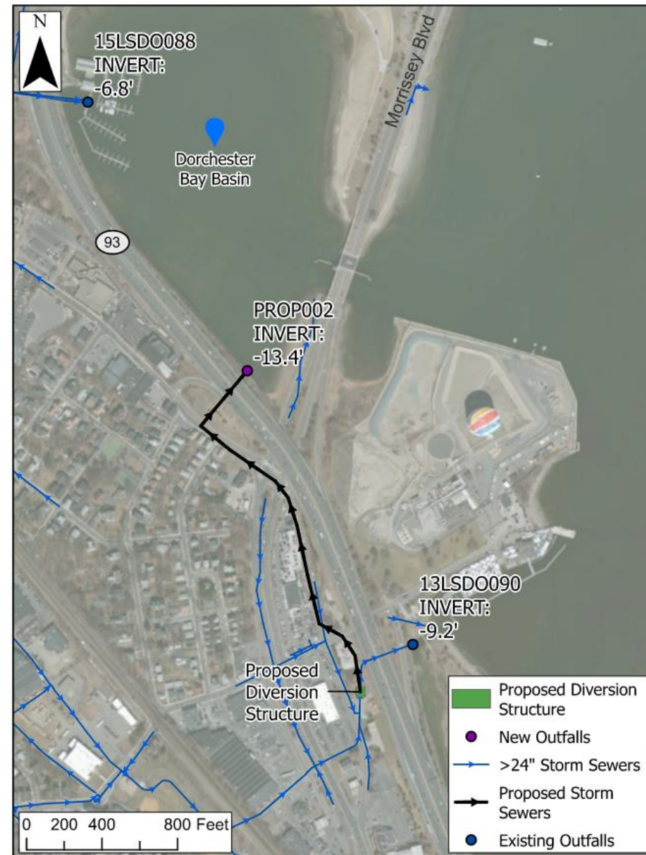
New pipeline to direct flow from 13LSDO090 to the DBB
