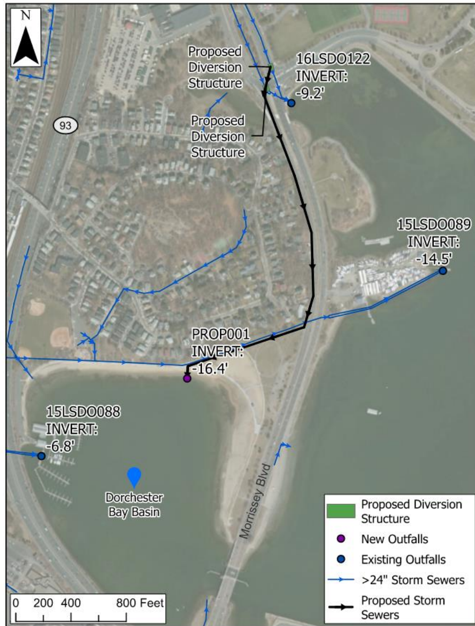
New pipeline to direct flow from 16LSDO0122 to the DBB
